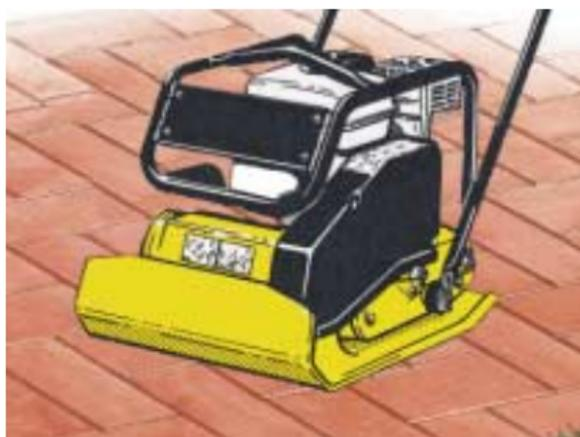
by placing two large screwdrivers in the joints on opposite sides of the paver and pry and rock it straight up. Tamp the replacement pavers into place with the plate compactor.
